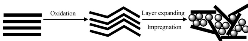
Fig. 1. Schematic illustration of Cu–Ni/graphite nanocomposite catalyst synthesis.
